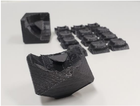
Figure 2.1 Rough surface of printed components due to the limited precision of the 3D printer
